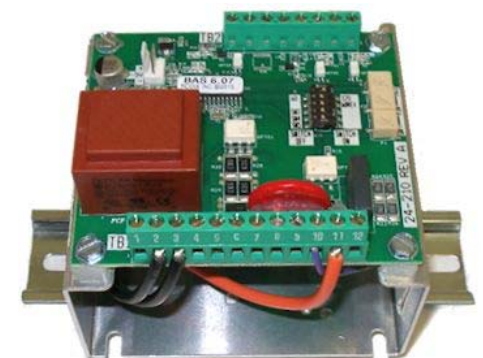
Bracket securely installed on DIN rail
